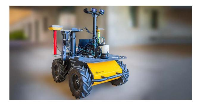
The base robot for the new plant-moisture-measuring system researchers are developing will navigate rows of crops to reach individual leaves and stems. Credit: University of California - Riverside
