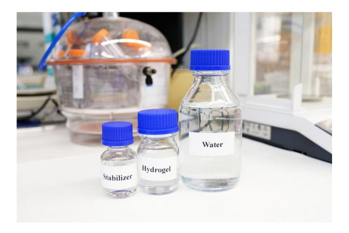
The liquid mixture used to create the smart window is made from microhydrogel, water and a stabiliser. Credit: NTU Singapore
