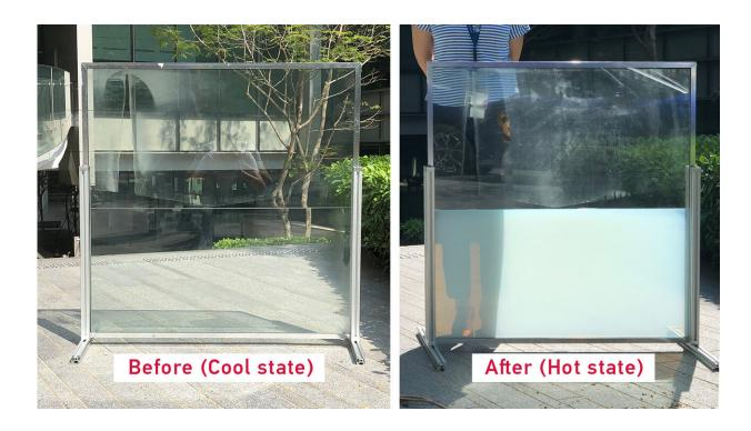
The smart window turns opaque when exposed to heat, thus blocking sunlight, and, when cool, returns to its original 'clear' state. Credit: NTU Singapore
