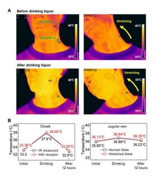
After attaching a sensor, the temperature changes of the ion-electronic skin before and after imbibing alcoholic drink was measured with an IR camera. The ion-electronic skin accurately recognizes body temperature despite the movement of the neck. Credit: POSTECH
