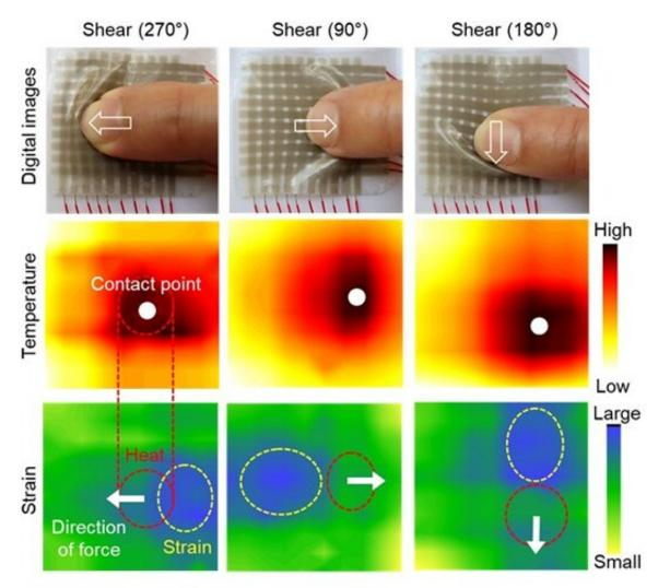
An image of recognition when the ion-electronic skin was pushed. The temperature change and direction of force in the part of contact are accurately recognized.
