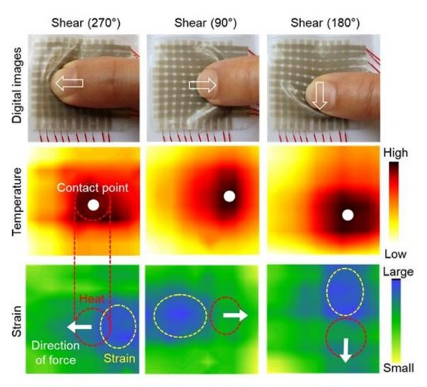
An image of recognition when the ion-electronic skin was pushed. The temperature change and direction of force in the part of contact are accurately recognized.
