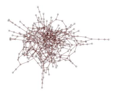
Image showing the nodes and lines of a prototypical power grid. It has a total of 400 nodes, of which 340 are nodes with only consumption, while the remaining 60 have consumption and generation. The nodes are interconnected by 617 lines. Credit: B. Carreras using Mathematica
