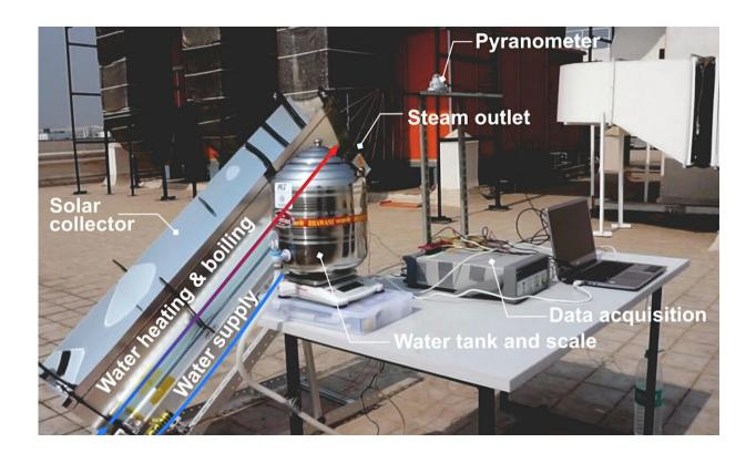
Autoclaves, which are used to sterilize medical tools, require a steady supply of hot, pressurized steam. Researchers at MIT and the Indian Institute of Technology have come up with a way to generate that steam passively, using just the power of sunlight, to help maintain safe, sterile equipment at low cost in remote locations. This photo shows an example of the new autoclave developed by researchers. Credit: Courtesy of the researchers. Edited by MIT News.
