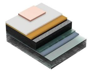
The planar p-i-n device architecture of the perovskite solar cell employed in the study. Credit: KAUST
