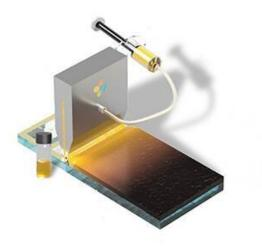
Slot-die coating technique used for large-scale fabrication of perovskite solar cells. Credit: KAUST
