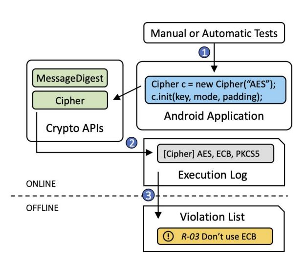
How Crylogger works: 1. CRYLOGGER runs the application with an instrumented crypto library.2. CRYLOGGER collects a log containing the parameters of the crypto API calls. 3. CRYLOGGER checks the crypto rules and reports all the violations. Credit: Luca Piccolboni/Columbia Engineering
