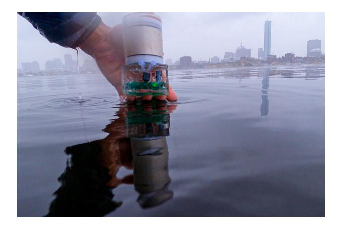
MIT researchers have built a battery-free pinpointing system dubbed Underwater Backscatter Localization (UBL). This photo shows the battery-free sensor encapsulated in a polymer before it is dipped into the Charles river. Credit: Reza Ghaffarivardavagh
