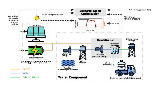
The water-energy nanogrid. Electricity generated at solar panels during peak availability is used to run a water nanofilteration system. Any excess energy is either fed to the battery pack or is available for basic household use. Credit: Dr. Le Xie and Dr. Shankar Chellam/Texas A&M University College of Engineering
