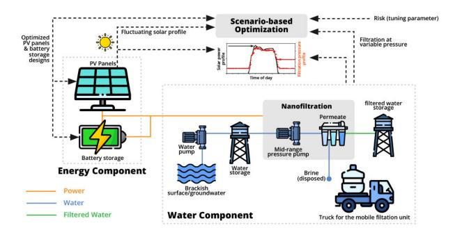
The water-energy nanogrid. Electricity generated at solar panels during peak availability is used to run a water nanofilteration system. Any excess energy is either fed to the battery pack or is available for basic household use. Credit: Dr. Le Xie and Dr. Shankar Chellam/Texas A&M University College of Engineering
