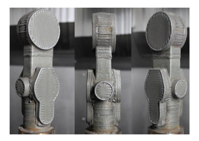
Compared with traditional metal additive manufacturing, this process contains multiple printable volumes that started from different building surfaces with different orientations. Credit: Xinyi Xiao, Penn State
