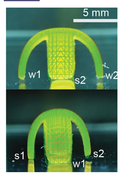
Bending the hybrid hydrogel with light resulted in a walking robot. Credit: Li et al., Sci. Robot. 6, eabb9822 (2020)
