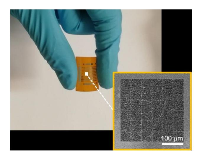
The quasi-2DEG photonic synapse device can be made on polyimide substrate and become flexible. Inset shows the corresponding SEM image of the fabricated  $6 \times 5$  device array. Credit: You Meng, City University of Hong Kong
