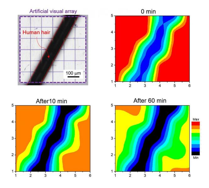
Researchers carry out experiments to test the artificial visual system. The figure on the top left hand corner shows a human hair was used to pattern the light. The other three figures show the imaging and memorizing behaviours of the artificial visual system after different retention time. Credit: *Science Advances* 10.1126/sciadv.abc6389
