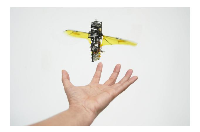
KUBeetle-S robot with the foldable wings. Credit: H. Vu Phan
