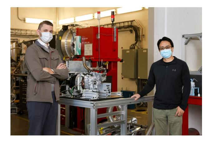
ORNL researchers Martin Wissink (L) and Ke An (R) worked with colleagues to design and test a running combustion engine prototype in the VULCAN beamline at the Spallation Neutron Source at ORNL, proving a new, non-destructive capability to analyze materials for advanced vehicles at the atomic level in a realistic setting. Credit: Genevieve Martin/ORNL U.S. Dept. of Energy.
