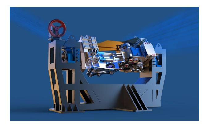
Oak Ridge National Laboratory is designing a neutronic research engine to evaluate new materials and designs for advanced vehicles using the facilities at the Spallation Neutron Source at ORNL. Credit: Jill Hemman/ORNL, U.S. Dept of Energy, and the Southwest Research Institute.
