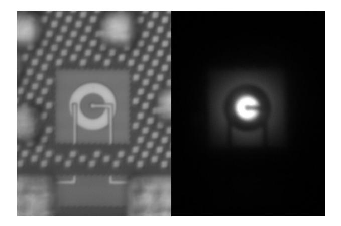
These two images show the silicon LED switched on (left) and off. Credit: Courtesy of the researchers
