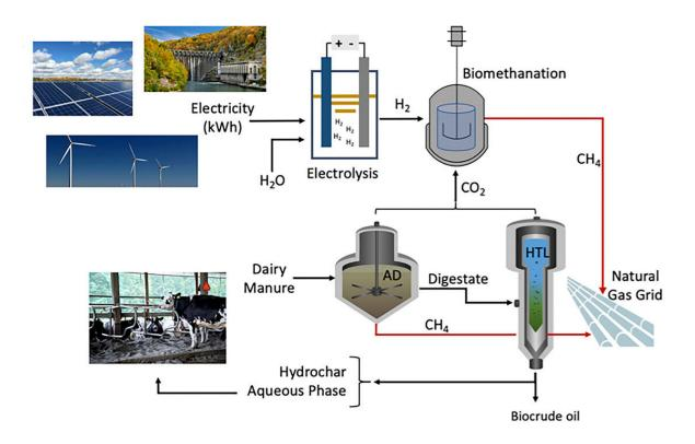
An integrated biorefinery approach utilizing agriculture waste biomass to produce renewable biomethane along with other co-products (for soil amendment, nutrient recovery, and transportation biofuels). Credit: Nazih Kassem, with images from Cornell University, Department of Energy
