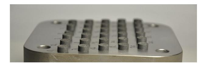
Developed under the 3DREMAG project, these magnets were 3D-printed from Nd-Fe-B powder. Credit: VTT
