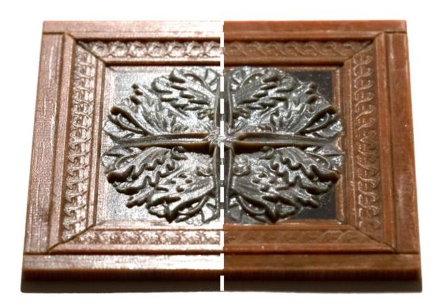
In this image, the left side shows traditional 3-D printing, which doesn't have varying reflectivity. The right side shows the new improvements, where one can choose which surfaces are glossy and which are matte. Credit: Massachusetts Institute of Technology
