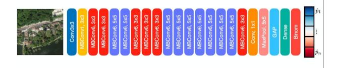
Model Architecture: The researchers' model takes the aerial tile as an input, which is then fed through several MBConv blocks. The feature maps end up going through a global average pooling layer and a dense layer to output a single value p. From it, probabilities for each socioeconomic class are generated from a binomial distribution. Credit: Abitbol & Karsai.
