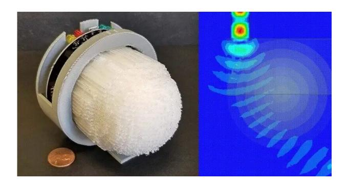
UD researchers are developing novel device lenses for wireless communications with the ability to bend communications signals. The project is collaborative with DeLUX engineering and leverages 3-D printing technology capabilities in UD's Additive Manufacturing Technology Center. Credit: University of Delaware
