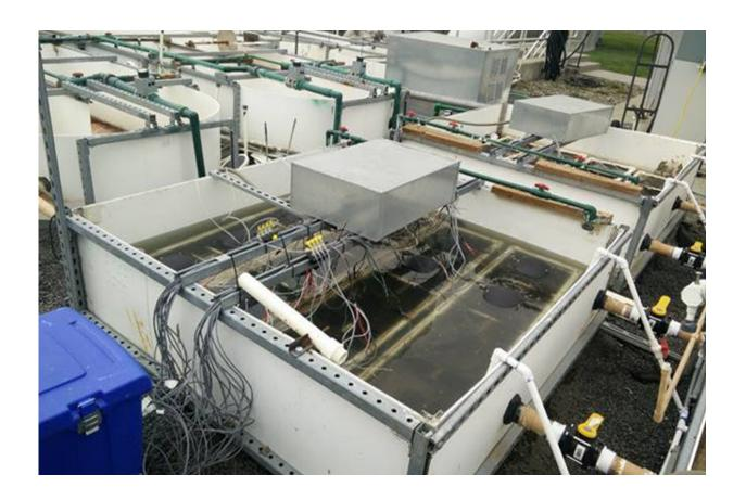
A switchable bioelectrochemical wastewater treatment system was tested at the pilot scale at a wastewater treatment facility in Moscow, Idaho. Credit: Washington State University
