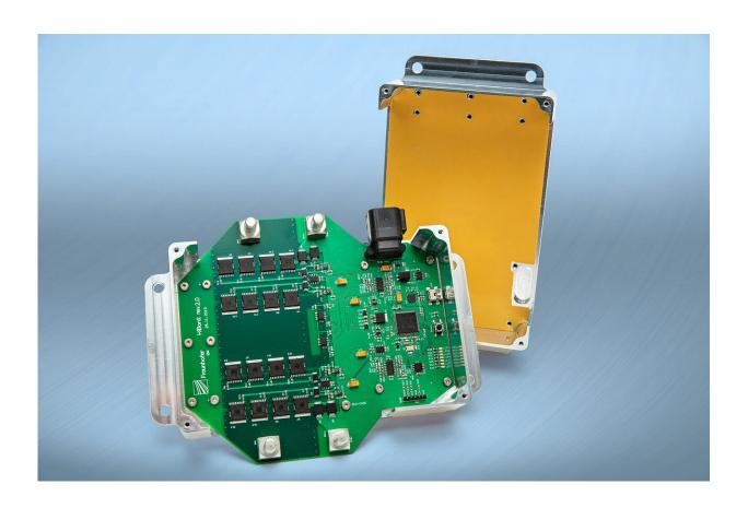
Developed by Fraunhofer researchers and partners, this new electronic module safeguards emergency operation in autonomous vehicles. Credit: Fraunhofer IZM/Volker Mai
