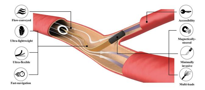
Schematic representation highlighting the features of flow-driven navigation. Hydrokinetic power is harnessed to propel syringe-injectable microscopic probes, ensuring autonomous navigation and obstacle avoidance. Magnetic fields provide steering to wirelessly access target daughter arteries. Credit: EPFL 2020
