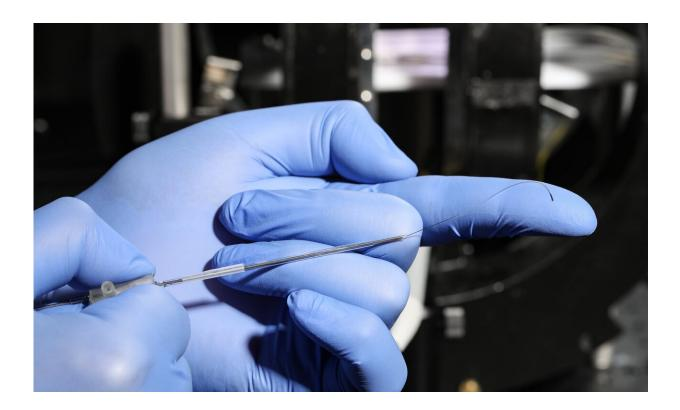
An ultraflexible endovascular flow sensor that is guided using magnetic fields. Credit: The photograph was taken by Alain Herzog/ EPFL 2020
