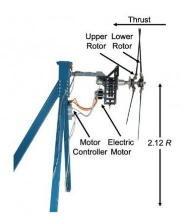
The test stand used during the experiment had the rotor shaft oriented horizontally to allow researchers to make acoustic measurements. Credit: U.S.
