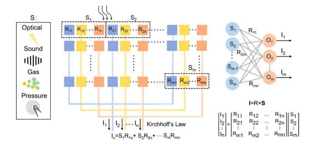
Schematic of in-sensor computing architecture with reconfigurable sensors for multiply-accumulation operations in the neural network. Credit: Zhou & Chai.
