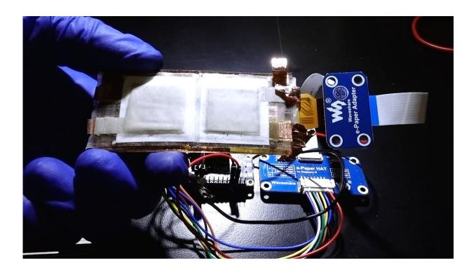
The batteries successfully powered a flexible display system equipped with a microcontroller and Bluetooth modules. Here too the battery performed better than commercially available Li coin cells. Credit: University of California San Diego
