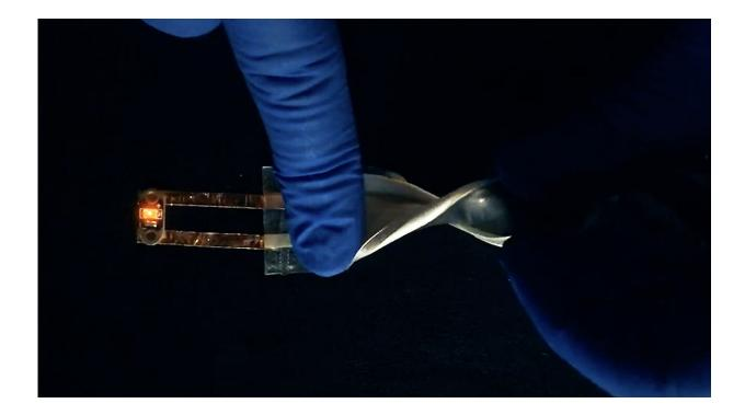
The areal capacity for this innovative battery is 50 milliamps per square centimeter at room temperature--this is 10-20 times greater than the areal capacity of a typical Lithium ion battery. So for the same surface area, the battery described in Joule can provide 5 to 10 times more power. Credit: University of California San Diego
