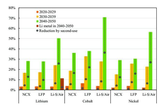
Closed-loop recycling potential of battery materials in periods of 2020–2029, 2030–2039, and 2040–2050 in the STEP scenario. Hydrometallurgical recycling is used for NCX and LFP batteries and mechanical recovery of Li metal for Li-S
