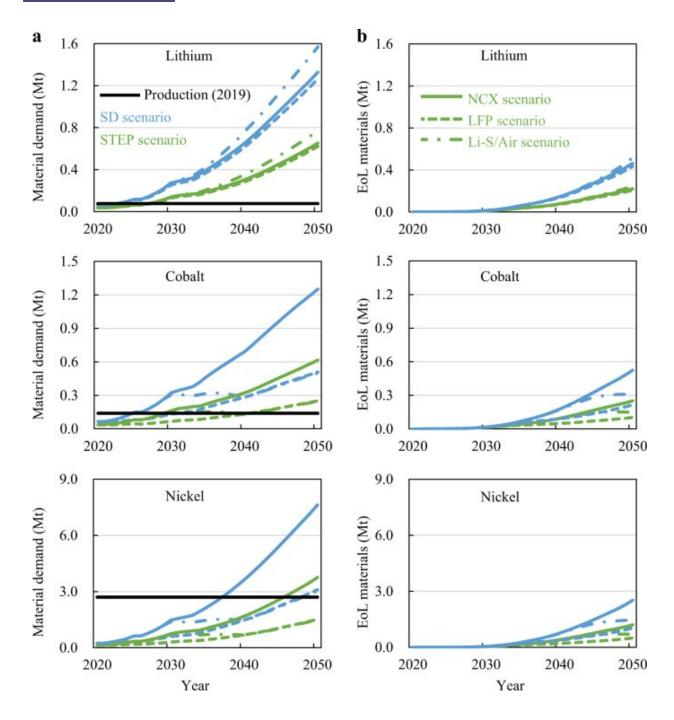
Battery material flows from 2020 to 2050 for lithium, nickel, and cobalt in the NCX, LFP, and Li-S/Air battery scenarios. (a) Primary material demand. (b) materials in end-of-life batteries. STEP scenario the Stated Policies scenario, SD scenario Sustainable Development scenario, Mt million tons. Credit: Nature Communications Materials, doi: 10.1038/s43246-020-00095-x
