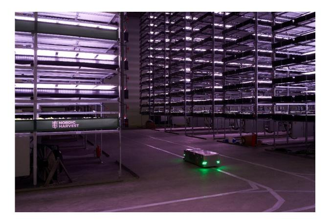
A robot, used to plant seeds and check the plants while growing, moves past vertical racks at 'Nordic Harvest' in Taastrup, a suburb west of Copenhagen
