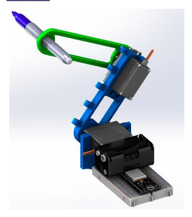
CAD render of the robotic arm assembly including the microcontroller and battery pack. Credit: Benitez et al.
