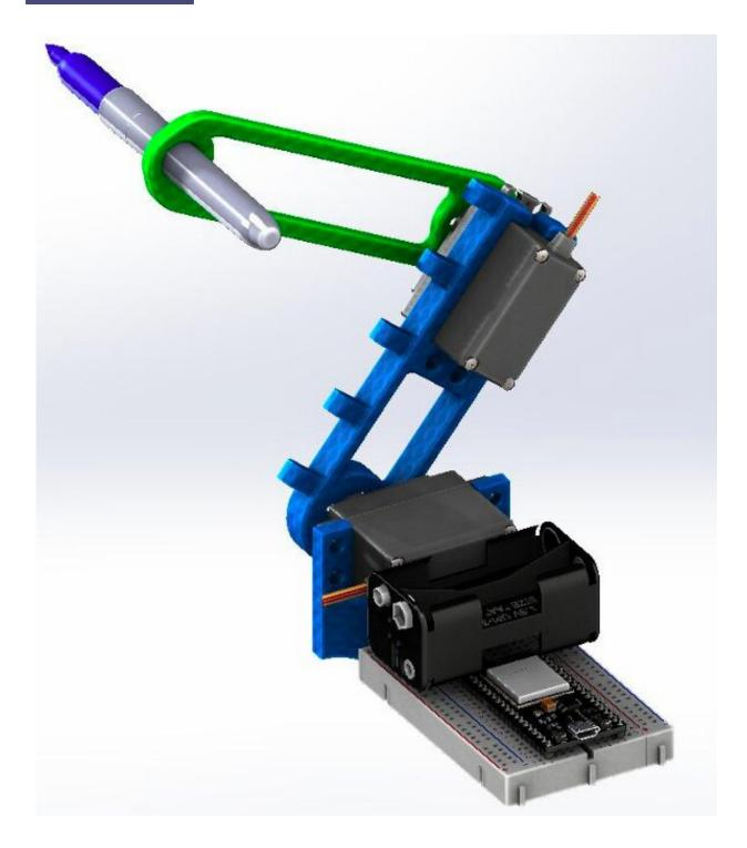
CAD render of the robotic arm assembly including the microcontroller and battery pack. Credit: Benitez et al.
