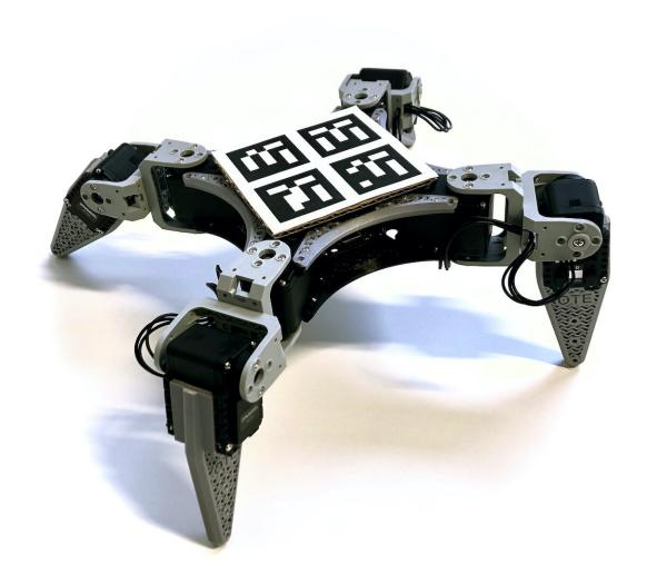
RealAnt: an open-source low-cost quadruped robot for real-world reinforcement
