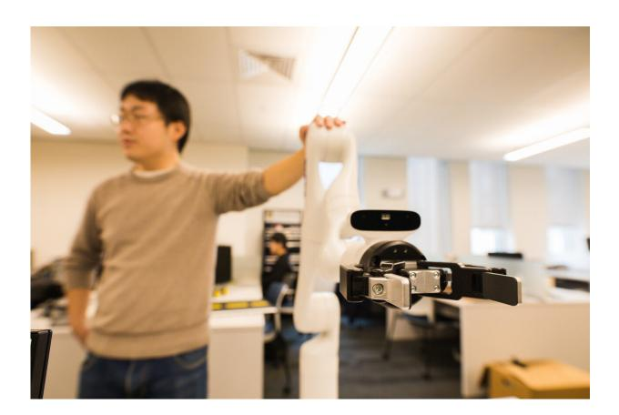
The team in Jeffrey C. Trinkle's lab work with a next-generation lightweight robotic arm designed specifically for academic and industrial research. A key feature of the arm, according to Jinda Cui, Ph.D. student and research assistant, is that it has "seven degrees of freedom," or seven independently controlled joints that allow for superior reachability in the three-dimensional workspace."This robot has one redundant joint that can move without impacting
