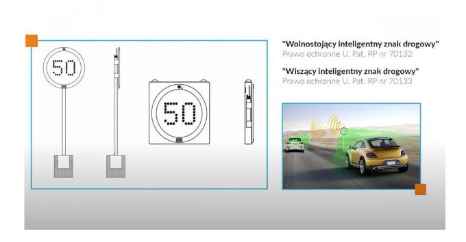
Researchers in Poland have created smart road signs that use built-in Doppler radar, video, and acoustic radar and weather stations to monitor road traffic and conditions to warn drivers in real-time of hazards and prevent collisions on highways. Credit: Czyzewski
