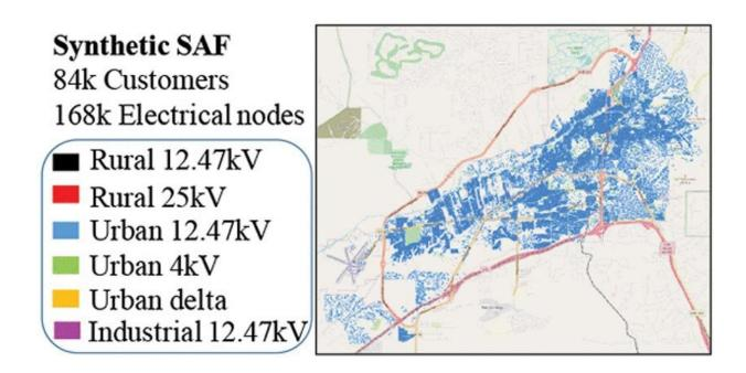
A Smart-DS synthetic distribution system dataset of Santa Fe, demonstrating Smart-DS' scale of grid representation. Credit: National Renewable Energy Laboratory
