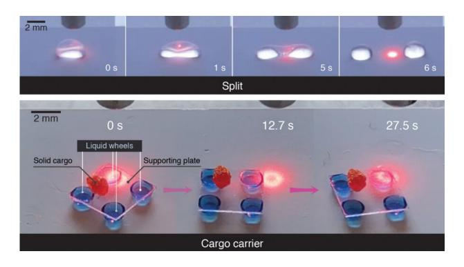
(upper photos) showing the split of an ethanol droplet by a beam of light on the photopyroelectric microfluidic platform.(below) showing a light-controlled cargo carrier with droplet wheels transporting a solid cargo. Credit: The University of Hong Kong
