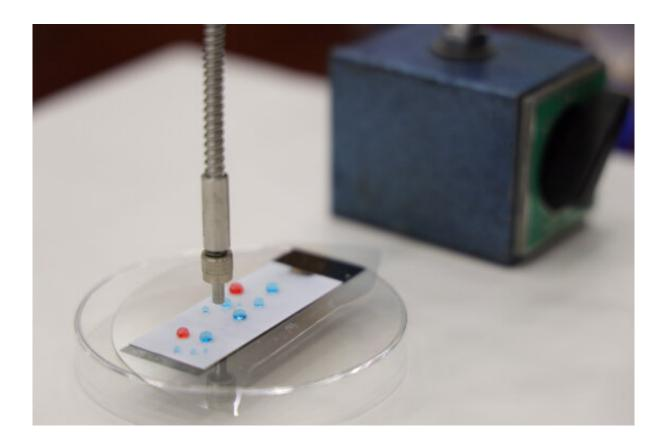
Demonstration of the light-controlled contamination-free fluidic processor. Credit: The University of Hong Kong
