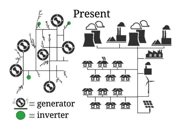
The present power system has historically been dominated by generators with large rotational inertia. Future power systems might have a significant fraction of inverter-based resources, which implies a need for next-generation controls to ensure stability. Credit: NREL
