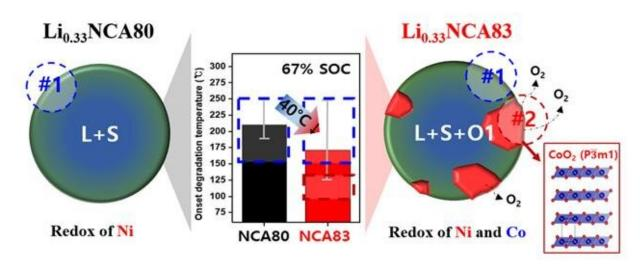
A graphical image depicting the role of an aluminum element that can reduce the risk of battery fires in NCA (nickel, cobalt, and aluminum), which is widely used as an anode material for electric vehicles. Credit: Korea Institue of Science and Technology(KIST)
