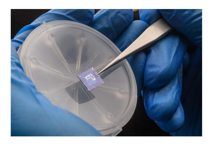
The four transistors on this chip were built out of a 2D material that disguises them from hackers. Credit: Purdue University /John Underwood
