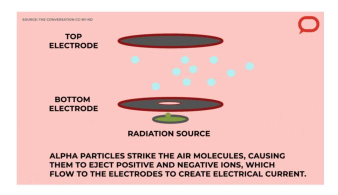
Alpha particles from the radiation source strike air molecules, which causes them to eject ions, creating a current. Credit: The Conversation
