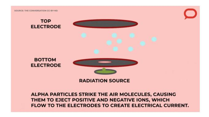
Smoke particles block the ions, stopping or reducing the flow of current, which sets off the alarm. Credit: The Conversation
