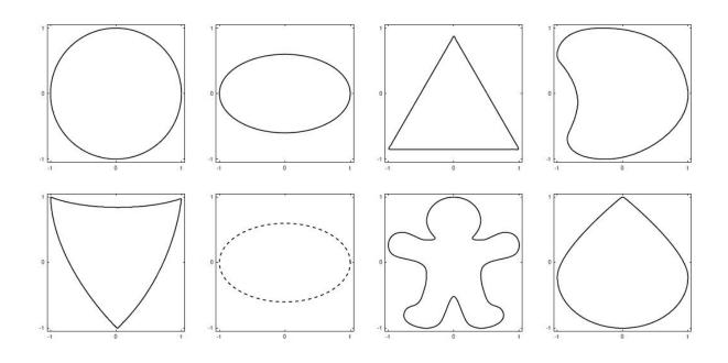
The electrosensing simulation's dictionary set, which contains seven shapes. The ellipse is repeated with a different electrical conductivity (represented by the dashed outline in the second row). Credit: Figure courtesy of Lorenzo Baldassari and Andrea Scapin.
