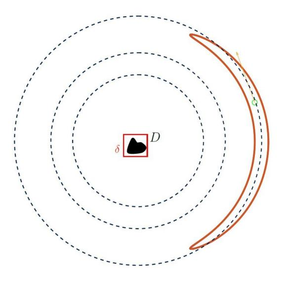
The simulated fish collects data about the target object (in the center) while swimming in multiple orbits at different length-scales (dotted lines). Credit: Figure courtesy of Lorenzo Baldassari and Andrea Scapin.
