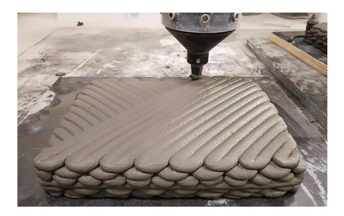
Concrete 3-D printed in patterns inspired by the internal structure of lobster shells. Credit: RMIT University
