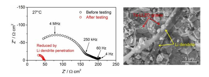
Nyquist plots of electrochemical impedance for Li/Ta-LLZO/Li symmetric cell before and after Li plating/stripping test (left) and Li dendrite penetration in Ta-LLZO (right). Credit: Toyohashi University of Technology.
