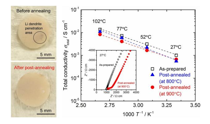
Photos of degraded Ta-LLZO by Li dendrite before and after post-annealing (left) and Li-ion conductivity of as-prepared and post-annealed Ta-LLZO (right). Credit: Toyohashi University of Technology.
