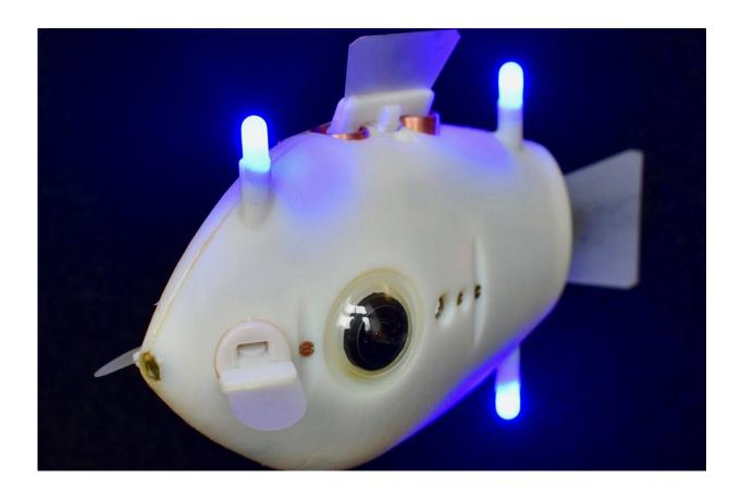
These fish-inspired robots can synchronize their movements without any outside control. Based on the simple production and detection of LED light, the robotic collective exhibits complex self-organized behaviors, including aggregation, dispersion and circle formation. Credit: Self-organizing Systems Research Group
