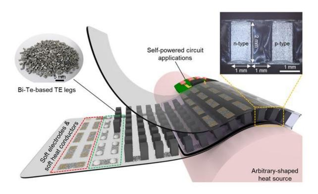
Conceptual illustration of a compliant TEG with soft electrodes and soft heat conductors (s-HCs) for self-powered circuit applications. The left inset is a photograph of bismuth telluride (Bi2Te3)-based thermoelectric (TE) legs and the right inset is an optical image of a cross-section of the compliant TEG. Scale bars, 5 and 1 mm. Credit: Korea Institute of Science and Technology (KIST)
