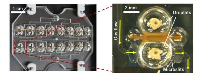
Photographs of the VOC sensor and one of the molecule exchange devices up close. Credit: © 2020 AAAS/Takeuchi et al.
