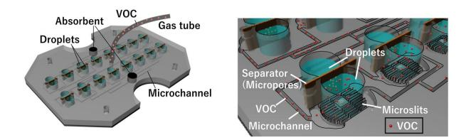
Schematic diagrams showing the network of tubes and channels that make up the VOC sensor. Credit: © 2020 AAAS/Takeuchi et al.
