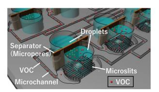
Schematic diagrams showing the network of tubes and channels that make up the VOC sensor. Credit: © 2020 AAAS/Takeuchi et al.
