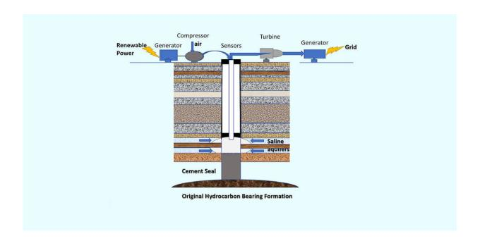
To store energy in idle wells, sustainable power created by solar panels and windmills placed near them would be converted into high-pressure air by a compressor. The air would travel through pipes to subsurface saline aquifers, or shallow wet sands, between 1,000 and 8,000 feet beneath the surface. The high-pressure air would remain safely underground until needed. Credit: Illustration/Iraj Ershaghi
