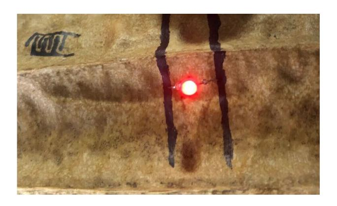
A pen containing conductive ink can draw circuits on a variety of surfaces -- even a loofah (seen here). Credit: Adapted from *ACS Applied Electronic Materials* 2020, DOI: 10.1021/acsaelm.0c00866
