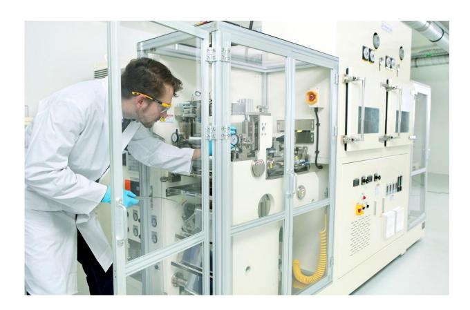
The coating of the electrodes is one of many process steps in complex battery cell production. Credit: WWU - MEET
