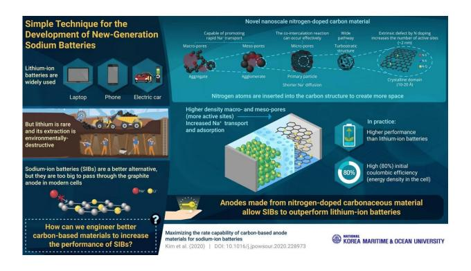
Researchers in Korea have developed a 'heteroatom-doped' (modified) carbon-based anode that helps sodium-ion batteries to surpass the performance of lithium-ion batteries. Credit: Korea Maritime and Ocean University
