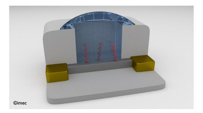
3D cross-section of a DNA (red) finFET biosensor of which the cavity in the oxide passivation layer enables liquid gating. Source and drain contacts are represented in gold. Credit: imec
