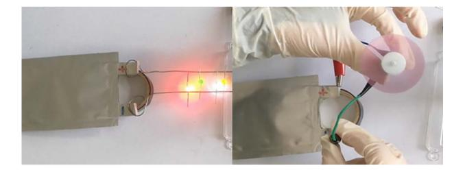
In Applied Physics Reviews, researchers in China describe how they applied basic physical concepts of atomic scale to build high-performance anodes for sodium-ion batteries. This image shows a homemade softpack sodium-ion battery they made. Credit: Jiangping Tu, Yuqian Li, Liyuan Zhang, Xiuli Wang, Xinhui Xia, Dong Xie, and Changdong Gu
